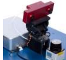
(g) Camera Videre STOC + Pan-Tilt + Hokuyo URG Laser
