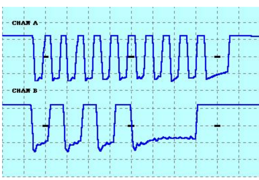
Figure 3: Scan code for the "Q" key (15h) being sent from a keyboard to the computer. Channel A is the Clock signal; channel B is the Data signal.
