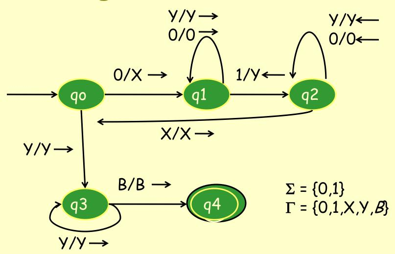
$$M = (\{q0,q1,q2,q3,q4\}, \{0,1\}, \{0,1,X,Y,B\}, \delta, q0, \{q4\})$$
