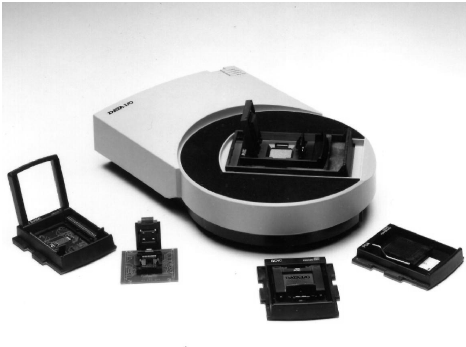
Figure 3.30. A PLD programming unit (courtesy of Data IO Corp).
