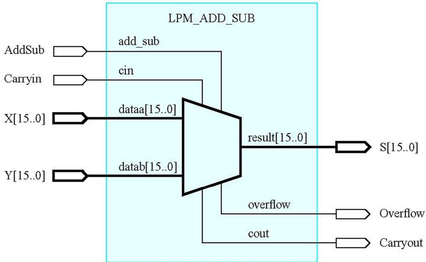
Figure 5.20. Schematic using an LPM adder/subtractor module.
