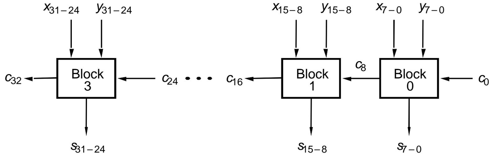
$$c_8 = g_7 + p_7g_6 + p_7p_6g_5 + p_7p_6p_5g_4 + \dots + p_7p_6p_5p_4p_3p_2p_1p_0c_0$$
