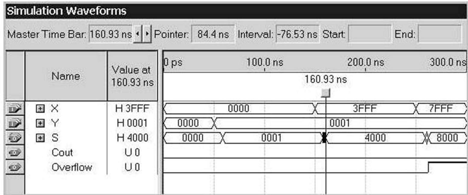
Figure 5.21. Simulation results for the LPM adder.
