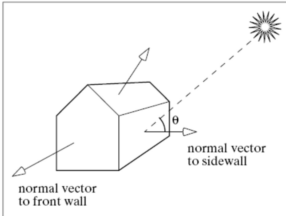
**FIGURE 6.2** The normal direction to a face determines its brightness.
