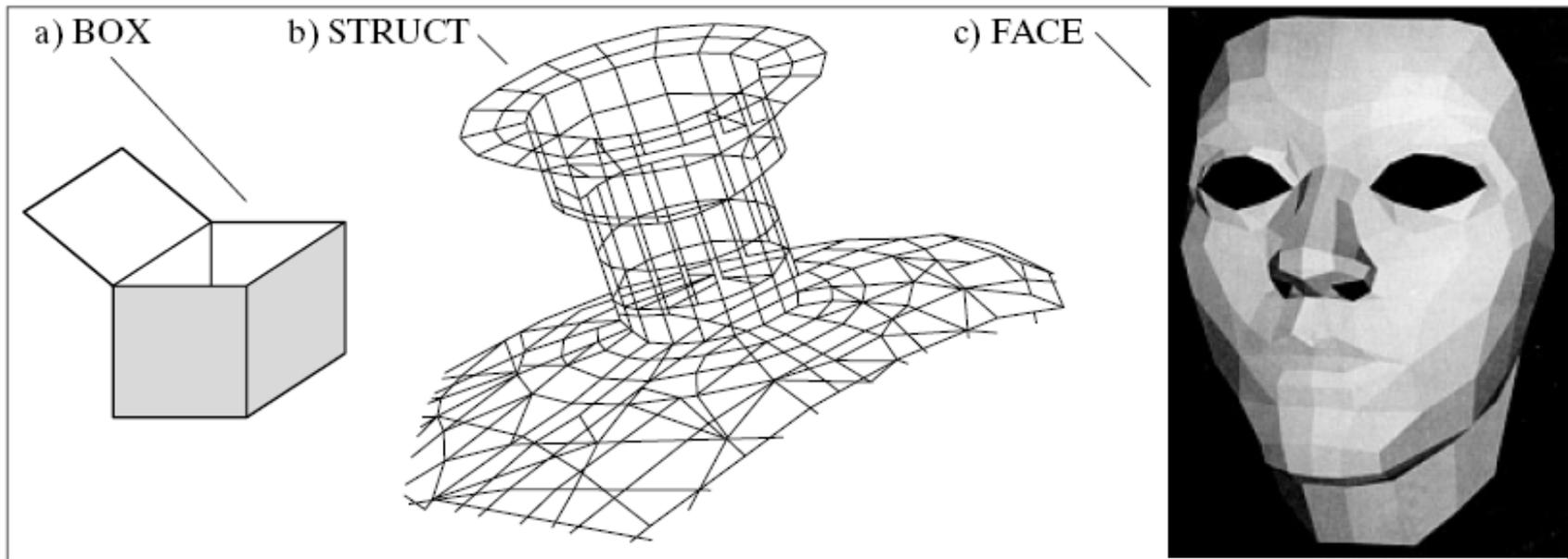
**FIGURE 6.12** Some surfaces describable by meshes. [Part (c) is courtesy of the University of Utah.]
