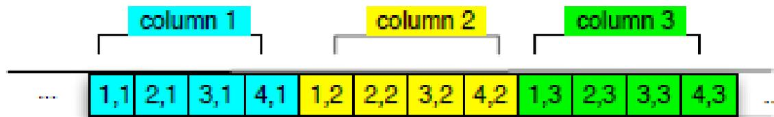
Figure 5: Column order storage for the array in Figure 3.
